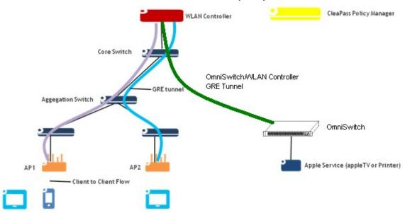
The mDNS feature is enabled on the OmniSwitch to support the mDNS service. A Layer 2 GRE tunnel interface is configured from the WLAN controller to the OmniSwitch to relay the mDNS messages. The mDNS message from the Bonjour capable wired service device is encapsulated and relayed from the OmniSwitch to the configured WLAN controller over the GRE tunnel. The WLAN controller then relays the mDNS messages received via the OmniSwitch GRE tunnel to the APs over the AP GRE tunnels.
