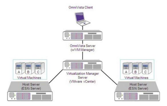
The diagram below provides a high-level view of an OmniVista/vCenter network configuration.
